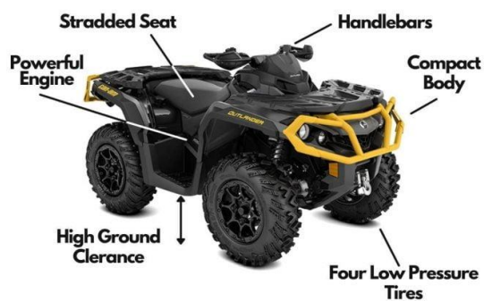
Figure 2. Main Features of All Terrain Vehicle
