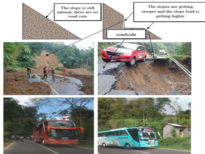
Figure 17. Illustration of Slope Change and Load Addition due to Slope Cutting, Heavy Vehicle Loads and Examples of Landslide Disaster Events;
