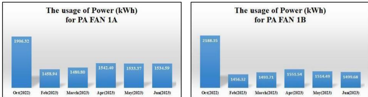
Figure 8. The average power consumption before and after the installation of the new APH element profile
