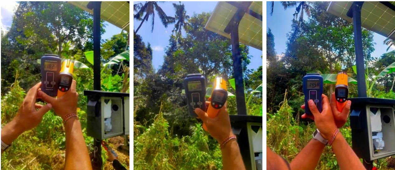
Figure 11. Irradiance and Solar Panel Temperature Measurement
